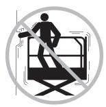
Do not modify or alter an aerial work platform. Mounting attachments for holding tools or other materials onto the platform, toeboards or guard rail system can increase the weight in the platform and the surface area of the platform or the load.
